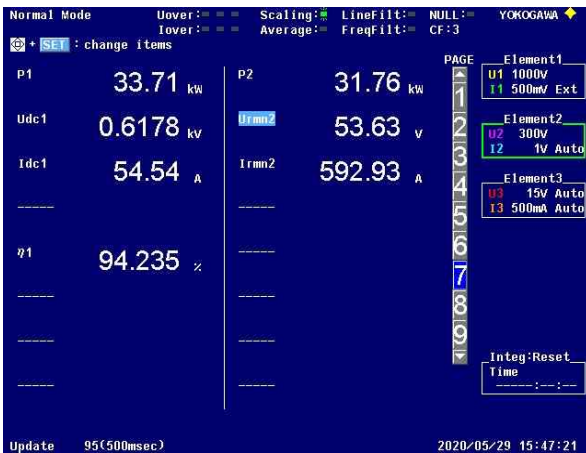
Fig. 10. Efficiency data of converter @30kW.
