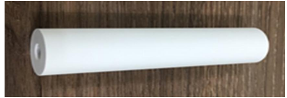
Fig. 3 Shape of ceramic insulator(green body)
