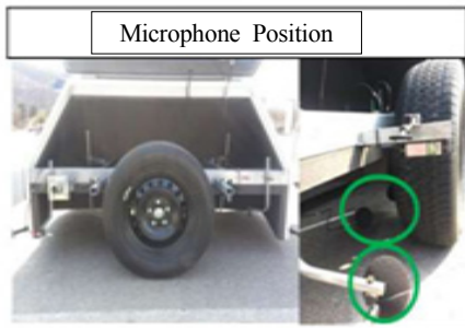
Fig. 6. Picture of Microphone in CPX Trailer
