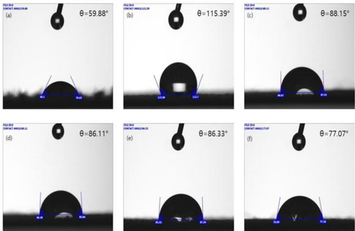
Figure 8. Contact angle of water droplets at 15% ODDMAC concentrations, curing(130°C, 10min) according to washing times; (a) untreated PET, (b) treated PET with 15% ODDMAC, (c) 5 times washing, (d) 10 times washing, (e) 25 times washing, (f) 50 times washing.
