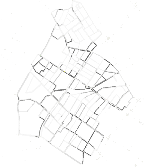
Fig. 2. Grayscale representation of link densities in the road network of Cologne at 8 a.m.
