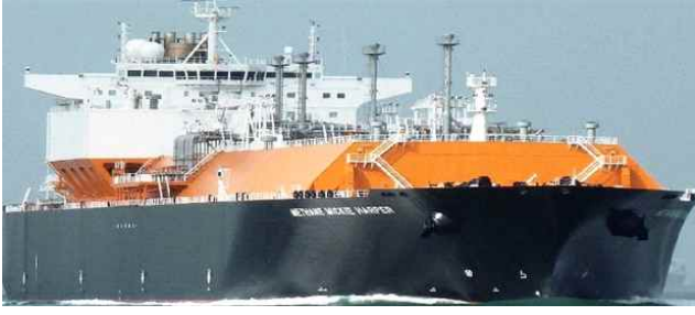
Fig. 1 170K Class LNG Carrier with air lubrication system (Kim et al., 2017)
