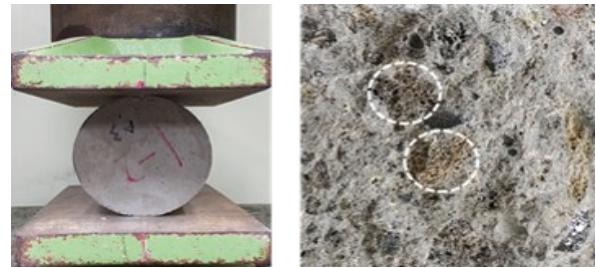
Fig. 7. Fracture of BAAC particles at the crack planes
