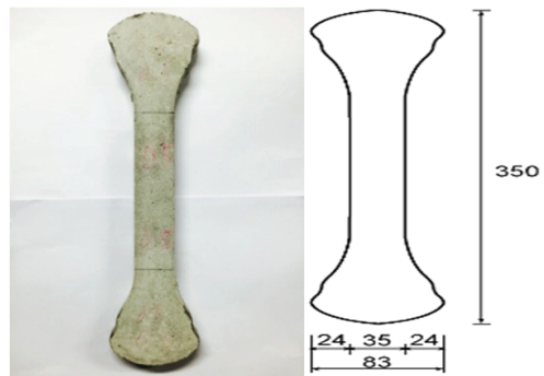
Fig. 1. Detail of specimen for direct tensile test
