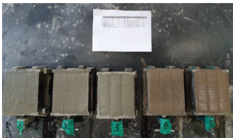
Fig. 1. The photos for placing the mortar containing mineral admixture in molds
