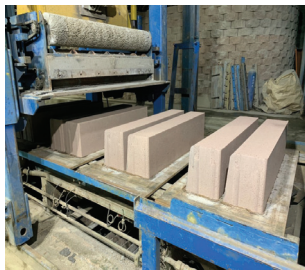
Fig. 1. The photo for production of mortar curbs
