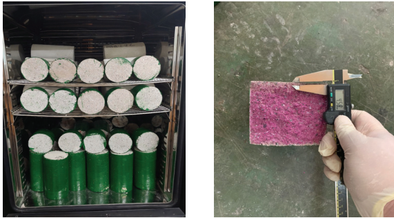
Fig. 5. The photos of accelerated carbonation test
