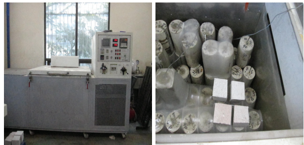
Fig. 4. The photos for freezing/thawing resistance performance test
