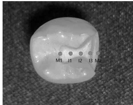
Figure 3. Measurement location of marginal (M1, M2) and internal area (I1, I2, I3).
