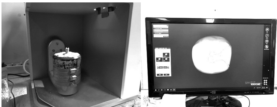
Figure 2. Scanning of mandibular lower first molar mesial occlusal cavity die and design of mesial occlusal cavity inlay.
