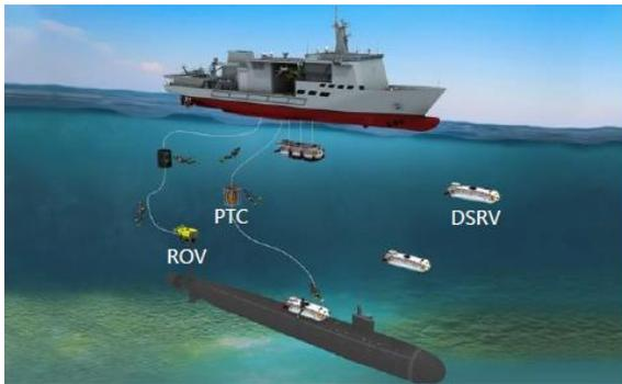
[Figure 2] Concept of operation of submarine rescue ship
