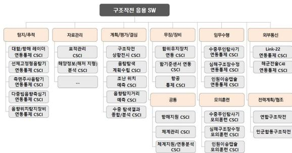
[Figure 11] Application S/W configuration of rescue operation system (draft)
