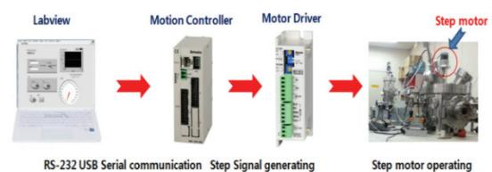
Fig. 3. The overview via the development of spin coater control system using stepmotor and LABVIEW software.
