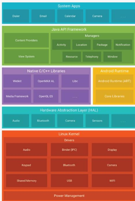
Fig. 1. Android Platform SW Stacks [9].
