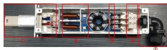
Fig. 5. High-impedance filter assembly photograph.
