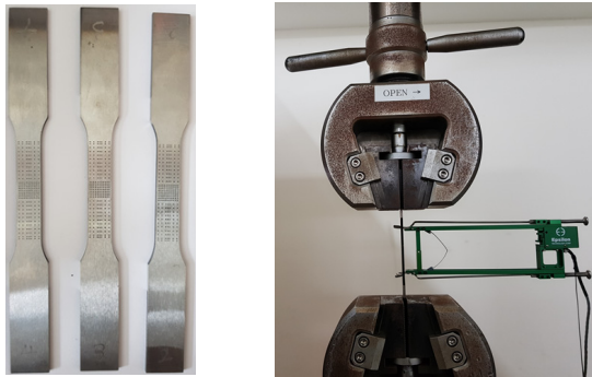
(a) Non-corroded Specimen (b) Test Set-up
