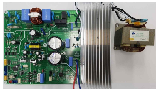
Fig. 11. Power converter for air conditioner compressor.
