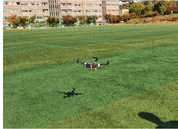
Fig. 9. Flight test for the quadrotor attitude control
