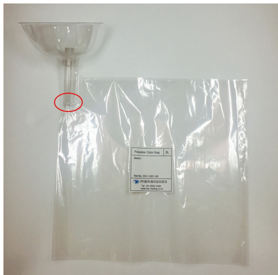
Fig. 1. Sample bag and location of deodorants. (part of the red circle ring)
