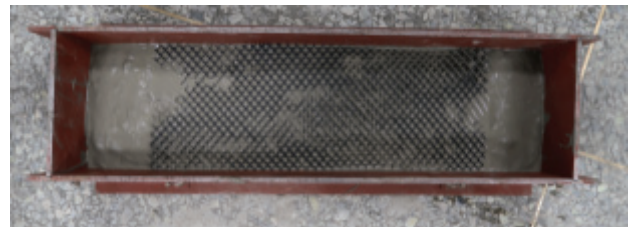
(b) Placing PE-mesh of Type-M7 specimen
