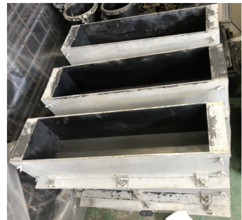
Fig. 2 Steel molds for flexural creep test specimens
