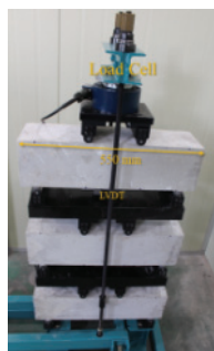
Fig. 5 Method of Flexural Creep
