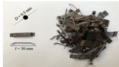
Fig. 1 Shape and appearance of fibers used in the SFRC
