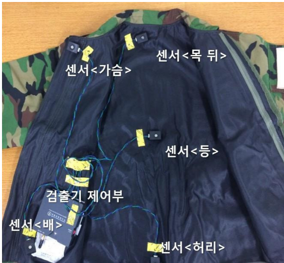
Fig. 14. Detecting point in protective clothing
