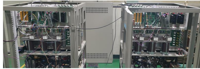
Fig. 5. Testing environment of parallel UPS.
