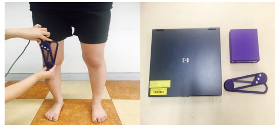
Fig 6. Electrogoniometer measurement and equipment
