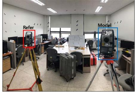
Fig. 3. Surveying of 3D points using total station
