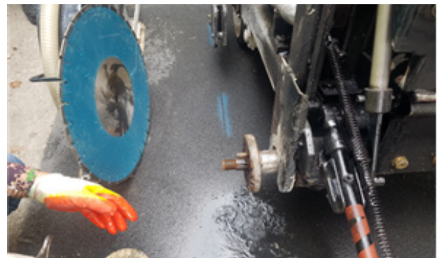
Fig. 15. Water spray inspection of eco-friendly road cutter
