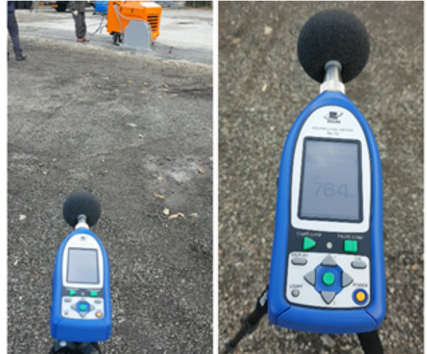
Fig. 19. Noise measurement scene caused by developed cutter
