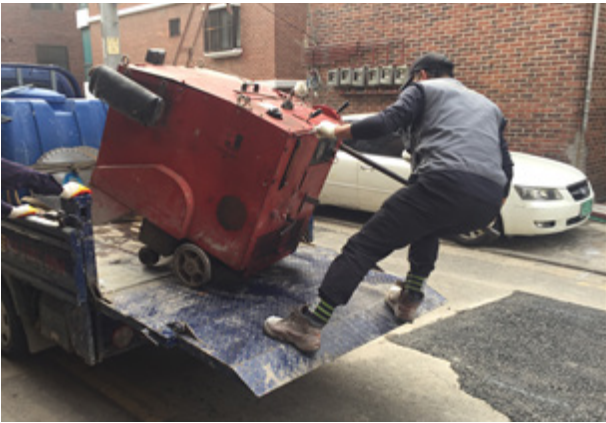
Fig. 6. Unloading Low Noise Road Cutter
