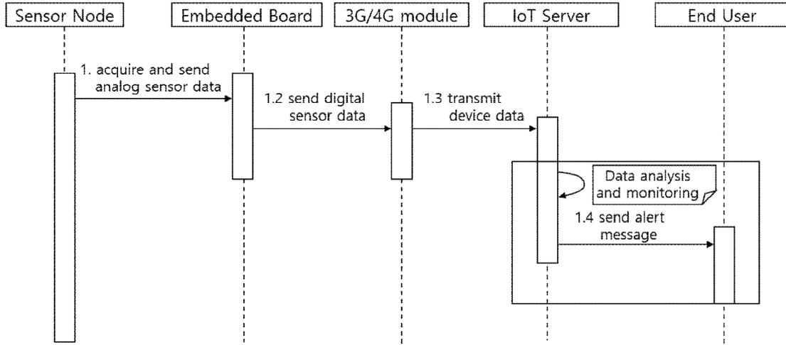
Fig. 6. Sequence diagram of system
