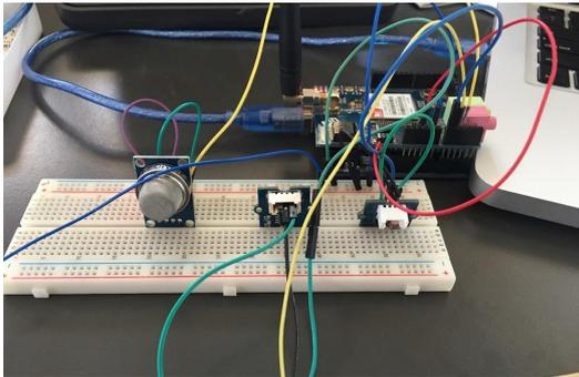
Fig. 8. Completed prototype for fire detection
