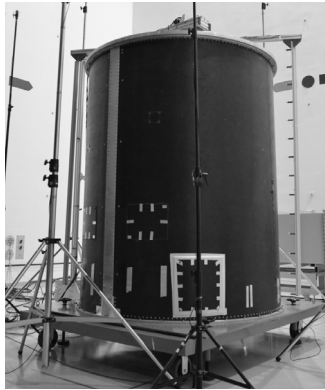
Fig. 10. Acoustic test for the cylinder part of Naro PLF.
