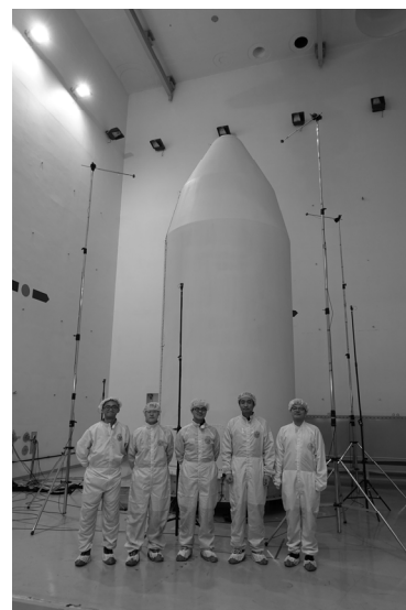
Fig. 14. Payload fairing (KSLV-II) acoustic test.
