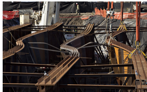
(b) Lateral torsional buckling
