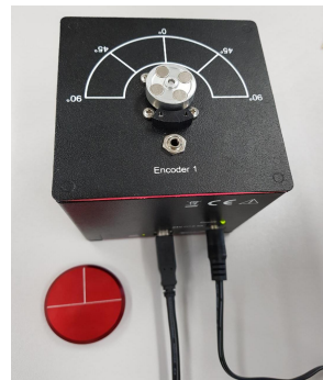
Fig. 2 Rotary motion control testbed: Quanser QUBE-Servo 2 system
