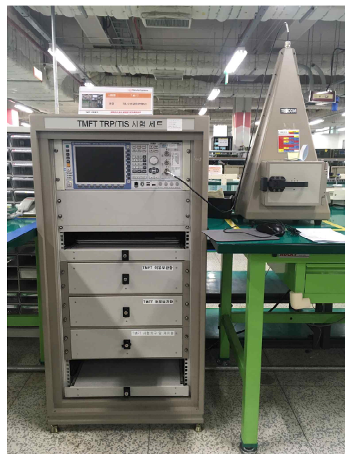
Fig. 3 TMFT TRP/TIS Test Equipment
