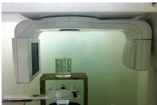
Fig. 2. SedentexCT IQ phantom is positioned for CBCT taking.
