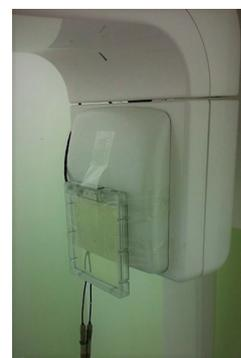
Fig. 1. Ionization chamber of DAP meter is located at the tube side of CBCT scanner for the DAP measurement.
