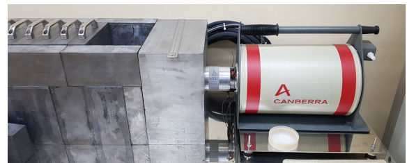
Fig. 3. Gamma-ray measurement spectrometer system (HPGe detector) of gamma-ray from the 179 Re sample.
