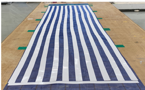
Fig. 5. Nylon Net with BOTDR Sensor
