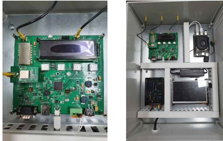
Fig. 4 The manufactured hardware of the module built in G/W.
