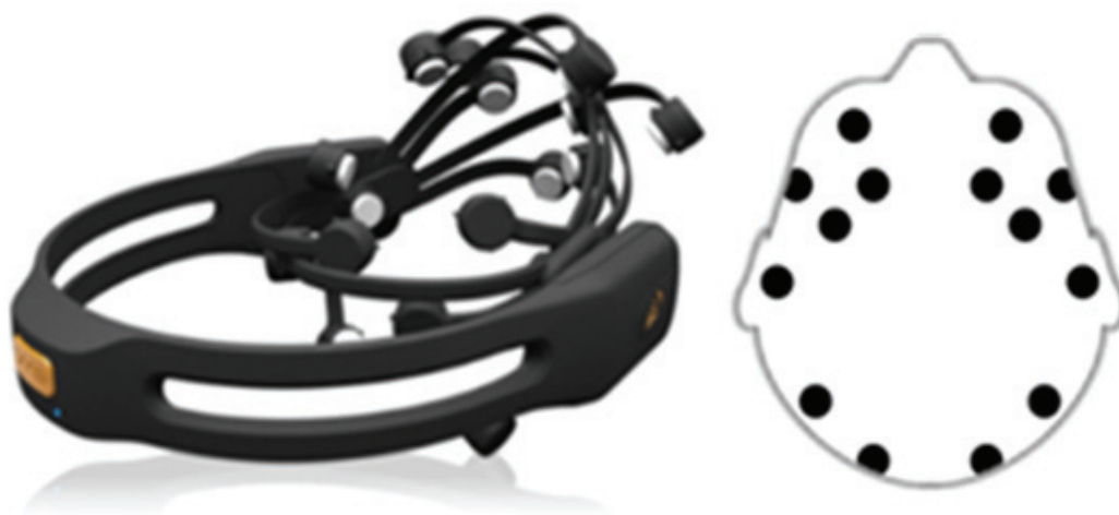
Figure 1. EEG measurement Instrument (EMOTIV Epoc ® + (EMOTIV, USA)).
