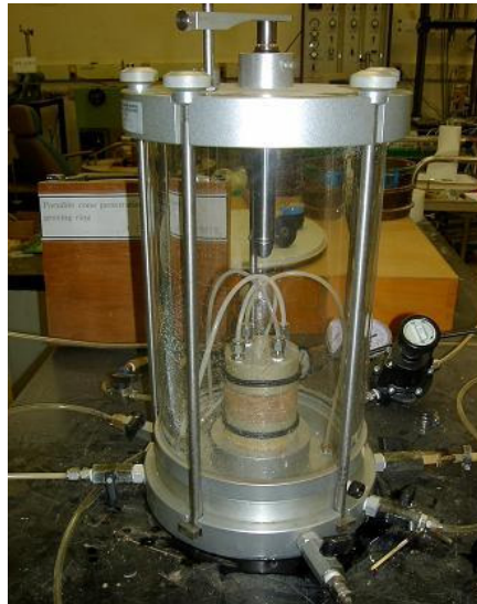
Fig. 2. Experimental apparatus for unsaturated permeability coefficient
