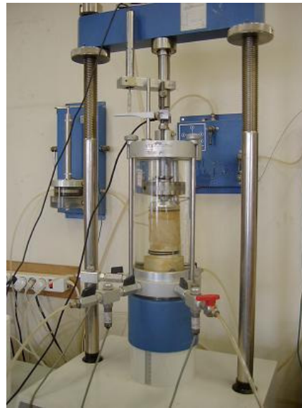
Fig. 3. Experimental apparatus for unsaturated shear strength
