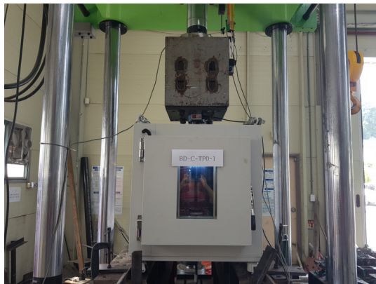
Fig. 1. Adhesion strength test set-up
