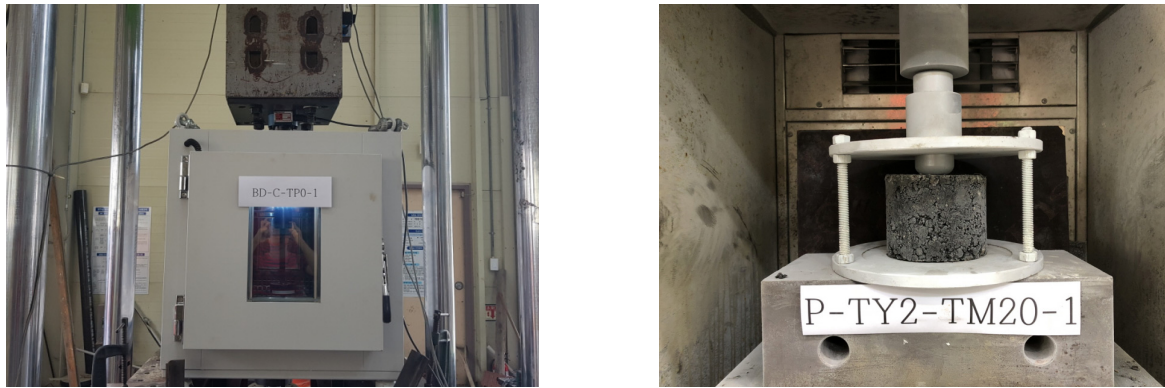
Fig. 2. Deformation strength test set-up
