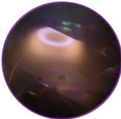
Fig. 3. Sputter plasma shape of pulse DC cathode.
