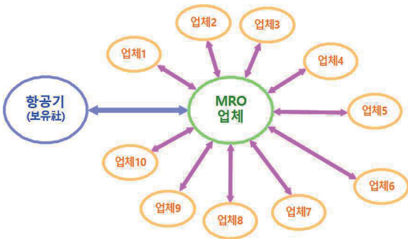
Fig. 1 Domestic Aircraft MRO Industrial Structure
