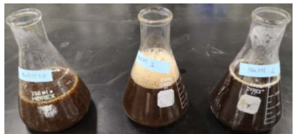
Fig. 4. From left to right, 0.1mol/L, 1mol/L and 2 mol/L feces and urine diapers solution after autoclave and filtration
