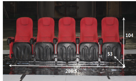
(a) Specimen of test 2 (Seat A, Unit : cm)
