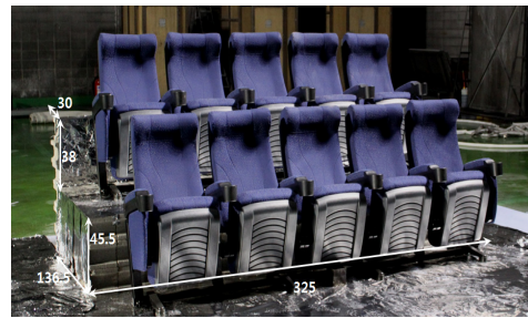
(b) Specimen of test 7 (Seat B, Unit : cm)
