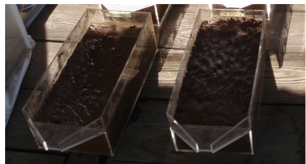
Fig. 2. Status of water drainage in the chambers before rainfall simulation (Left: control; Right: CMDS treated).
