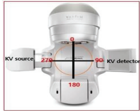
Fig. 2. The Rotation Coordinates for a Varian Linear Accelerator. 180° is a Reached through a Counterclockwise Rotation it is indexed as 180°E.
