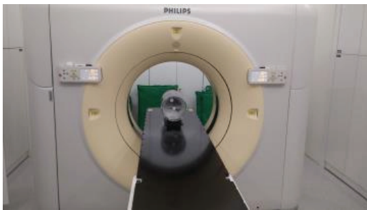
Fig. 1. Experimental Set-up of the AAPM CT Performance Phantom.
