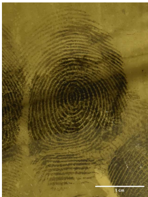
Fig. 9. Fingerprint on adhesive side of tape treated with Wet Powder Black ® . Fingerprints were photographed under white light.
