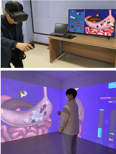
Fig. 3 Immersive virtual environments for education: HMD-typed VR environment(Top) and Multi-projection based environment(Bottom).
