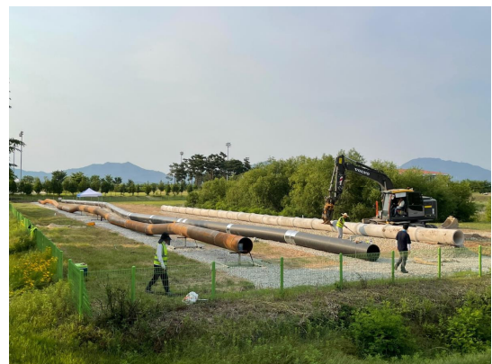
Fig. 3. Preparation for field test (steel, double-wall, con'c from the left)
