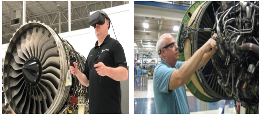
Fig. 1. Aircraft engine maintenance training with VR [1,8] and GE Aviation pairs Google Glass with smart wrench based on AR technology[1,9]
