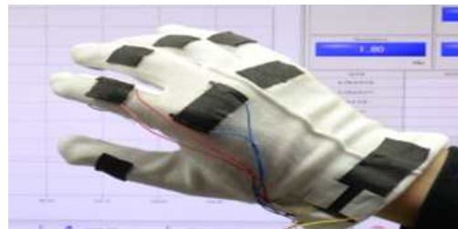
Figure 3. Graphene-based Textile Strain Pressure Complex Sensor Applied to Cotton Gloves to Detect Body Signals according to Hand Movements ( https://www.etri.re.kr )
