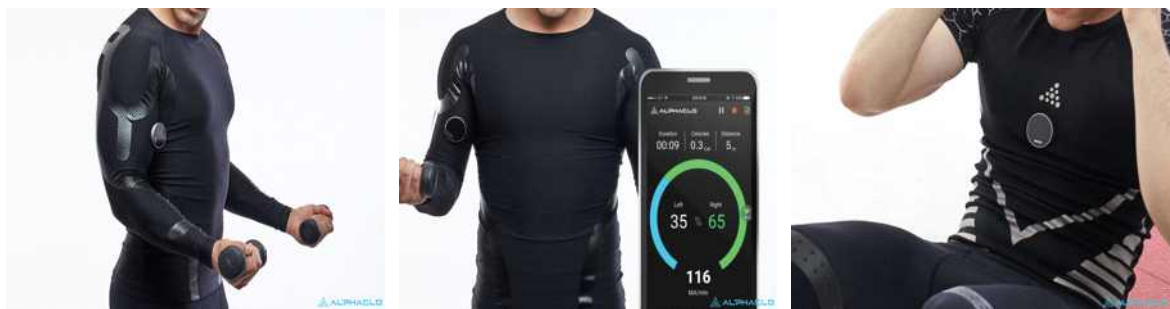
Figure 2. Muscle ware Technology for Correcting Posture by Attaching Stretch Sensors to Clothing ( https://www.facebook.com )
